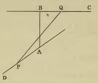
PA and QB are both perpendicular to AB, and therefore AB is the projection of PQ on AB, and is equal to the length of PQ multiplied by the cosine of the angle between them, and is therefore less than PQ, since the cosine of any angle is less than unity.
